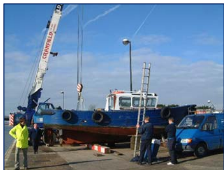
The RoDMA I workboat hoisted onto dry land for her biennial re-painting of the hull and superstructure.
